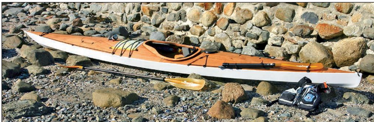
Finished and ready to go paddling, designer Bill Thomas's Willow kayak carries a compass and chart forward of the cockpit. A spare paddle rides on the afterdeck.
