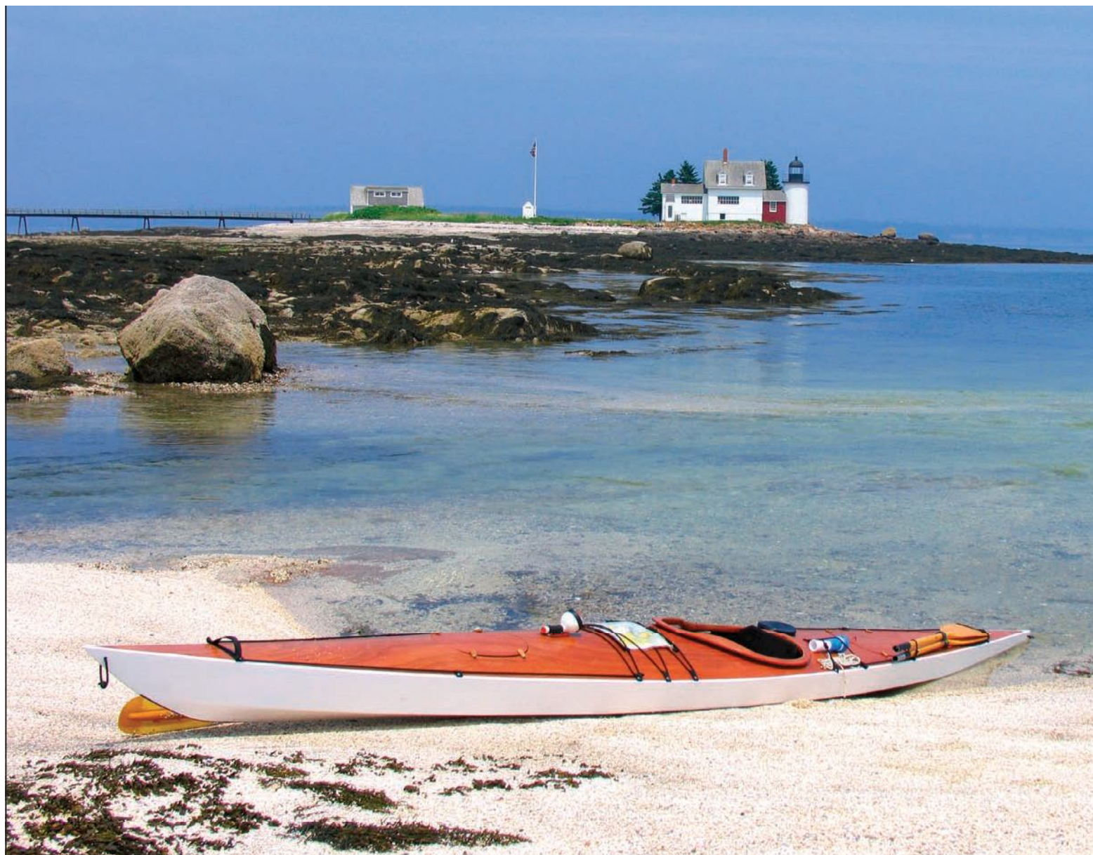
On a perfect Maine day in high summer, the Willow sea kayak rests on a beach near Green Island Light. Built stitch-and-glue fashion with high-quality plywood and epoxy, the 17'8" x 23" x 45-lb boat is tight and tough.
